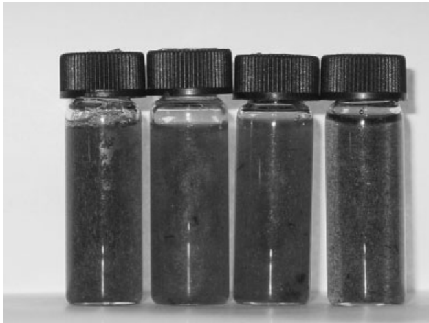
Figure 3 Optical photographs of Molau tests of the composites in formic acid. From left to right: PA6/20|CF/1|OMMT/1, PA6/20|CF/1|Na-MMT/1, PA6/20|CF/1|MICA/1, and PA6/20|CF/1.
