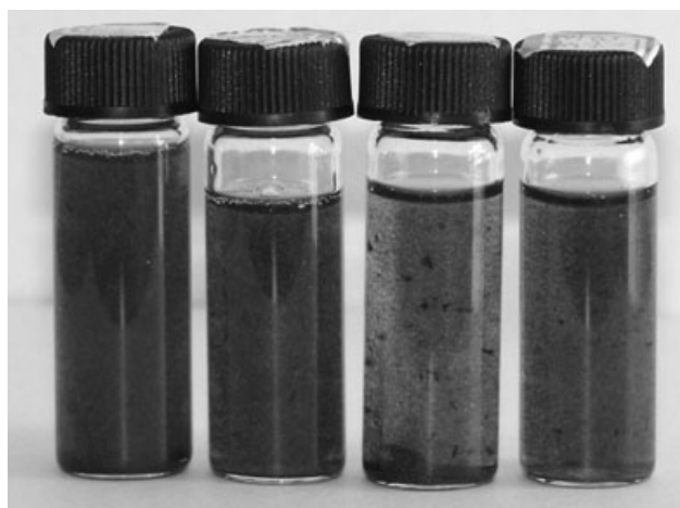
Figure 1 Optical photographs of Molau tests of the composites in formic acid. From left to right: PA6/20|CF/1|OMMT/1, PA6/20|CF/1|OMMT/0.4, PA6/20|CF/1, and PA6/20|CF/1. The treated CF is mixed for 10 min for the rightmost sample or 3 min for the others.
